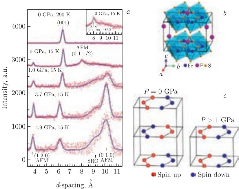
a) Neutron diffraction patterns of  $\text{FePS}_3$ , measured at selected pressures and temperatures and processed with the Rietveld method. b) Monoclinic structure of  $\text{FePS}_3$  with the  $C2/m$  symmetry. c) Magnetic structure of  $\text{FePS}_3$  at ambient and high pressures
