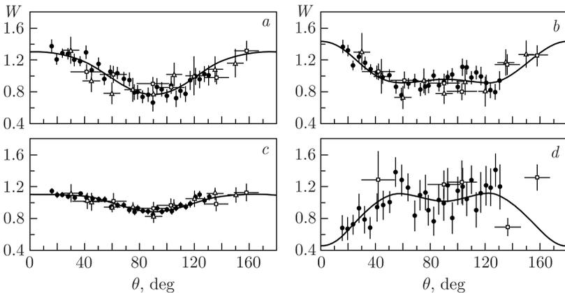
Angular distributions of  $\gamma$  quanta for  $E_\gamma = 935.5$  keV (a), 1333.7 keV (b), 1434.1 keV (c), and 1530.7 keV (d) transitions in the reaction  $^{52}\text{Cr}(n, n'\gamma)^{52}\text{Cr}$ . Solid curve — approximation of data by Legendre polynomials
