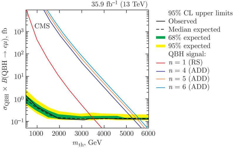
Upper limits at 95% CL for the mean value of the product of the signal cross section and the branching fraction for the QBH decay into  $e\mu$  as a function of the threshold mass  $m_{\text{th}}$ . 68% and 95% CL intervals for the median are shown by the inner green and outer yellow shadings, respectively. Predictions are also shown for several models with large extra spatial dimensions, in particular, for one extra dimension (RS) and for 4, 5, and 6 extra dimensions (ADD)
